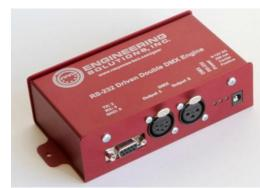
The protocol for the unit is all ASCII and easy to implement. Creating level control for the lights was easy to do and the response was quick. The following features are available with the unit:
