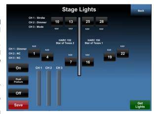
For recalling presets in a room, the module has room presets signal controls for up to 10 presets. These presets use the Start and End Mask values to recall only the channel values associated with the room.
